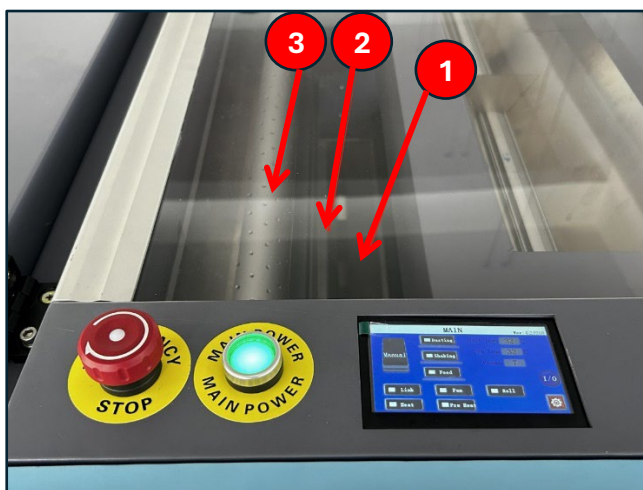
Master Power & Reset Switch. Has Lock-Out Function so the door panel will only open if the switch is in the OFF position.
